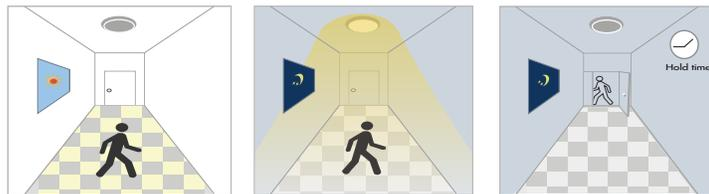
With sufficient daylight, even when motion is detected, light remains OFF.
